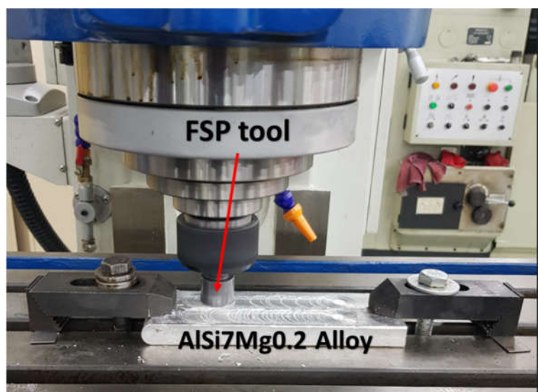
Figure 2. FS processing via an automatic milling machine.
